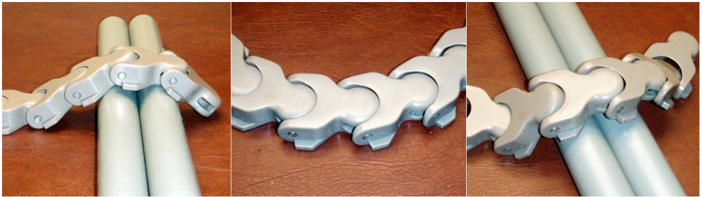
Figure 9 Conveyor Pivots Up/Down – Side to Side - Combined
