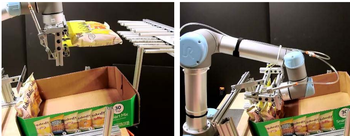
Figure 11 Alpha Robot Test Unit Grabbing Row of Bags and Loading into Case
