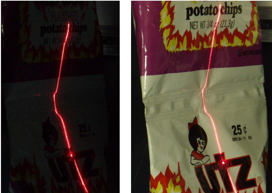
Figure 8 Image of Angled Projected Laser Line as Viewed by Camera
