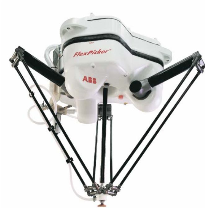
Figure 1b Delta configuration robot (Courtesy ABB)
