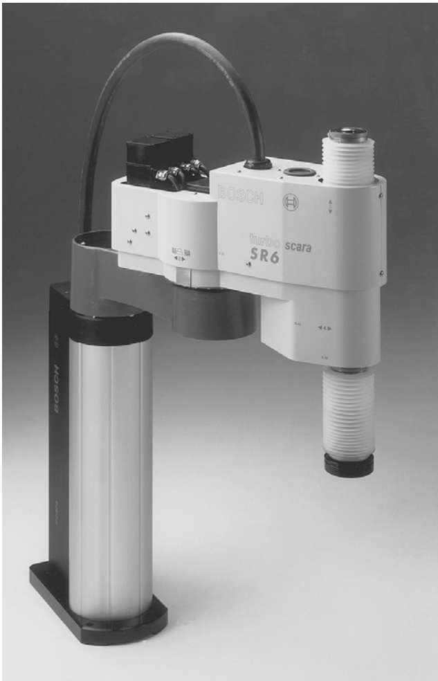
Figure 1a Standard SCARA robot (Courtesy Bosch)
