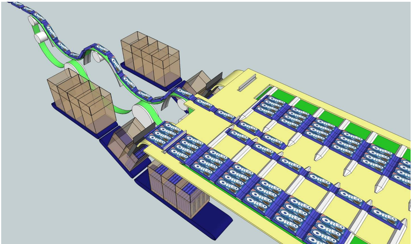
Figure 1 Exiting Embodiment of Case Packer Using Flex Conveyor for Timing Benefits
