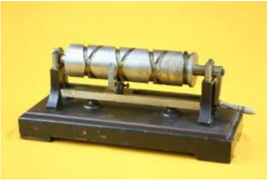
Figure 4 Reversing Helical Thread on a Barrel Cam
